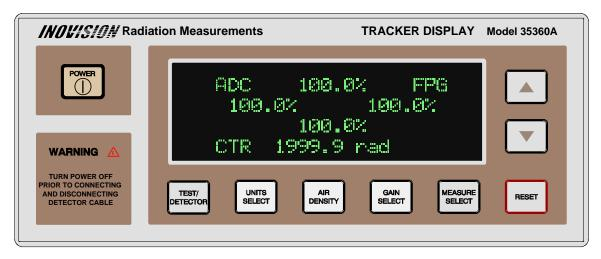
Figure 2-6. The Model 35360A TRACKER Display Front Panel
